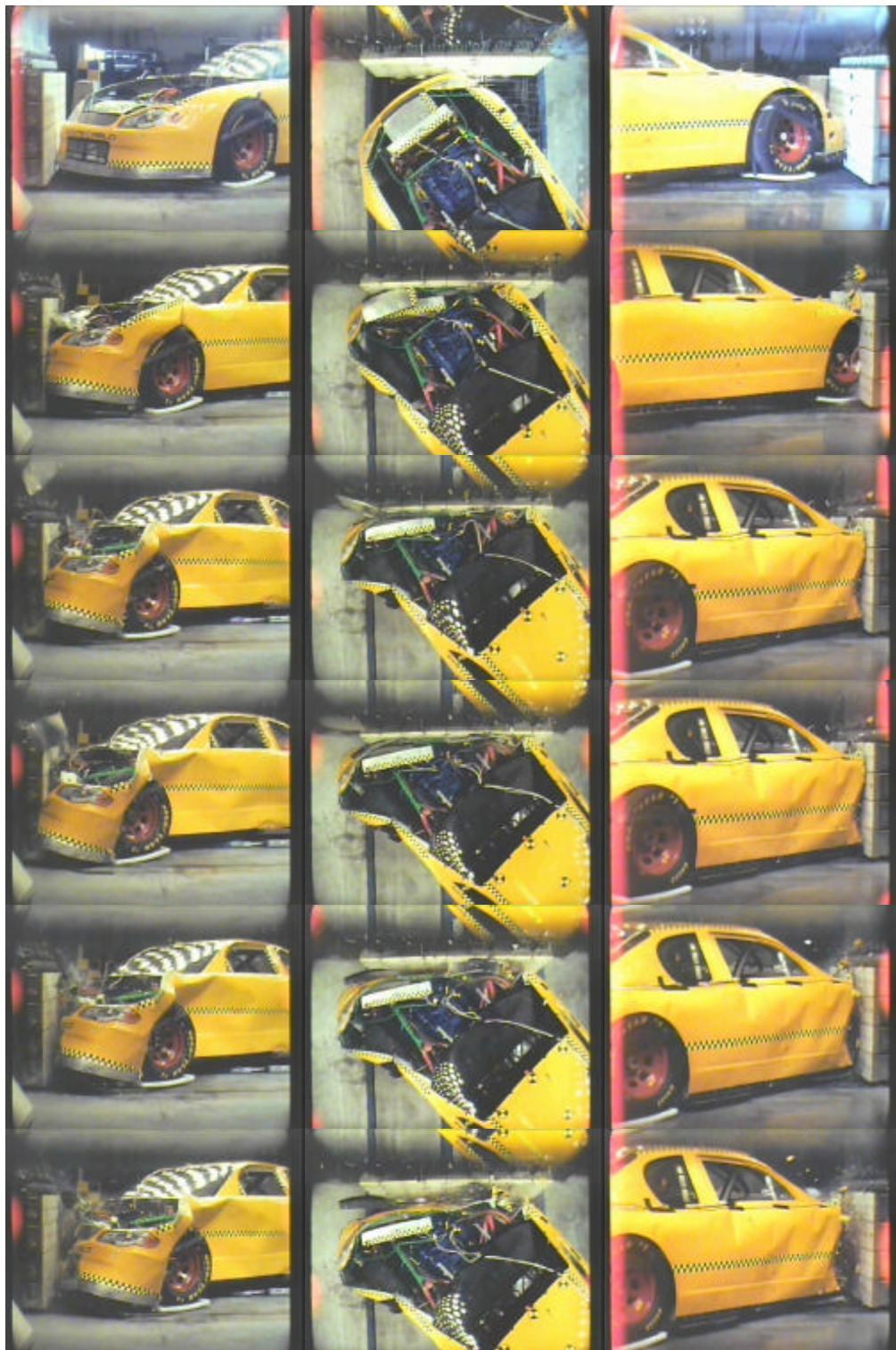
Figure 24. Sequential Photos from Full-Scale Crash Test
