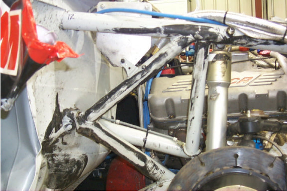
Figure 10. Structural Supports for Right Front Frame Rail.
