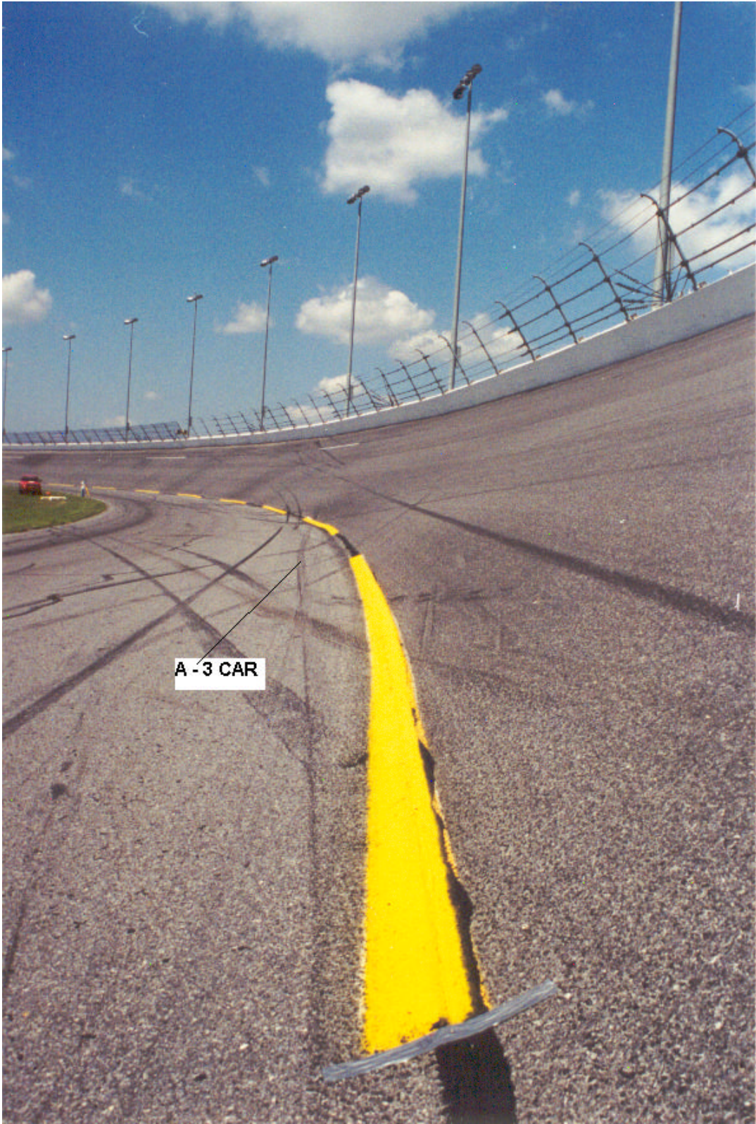
Figure 1. No. 3 Car Tire Mark Inside of Track
