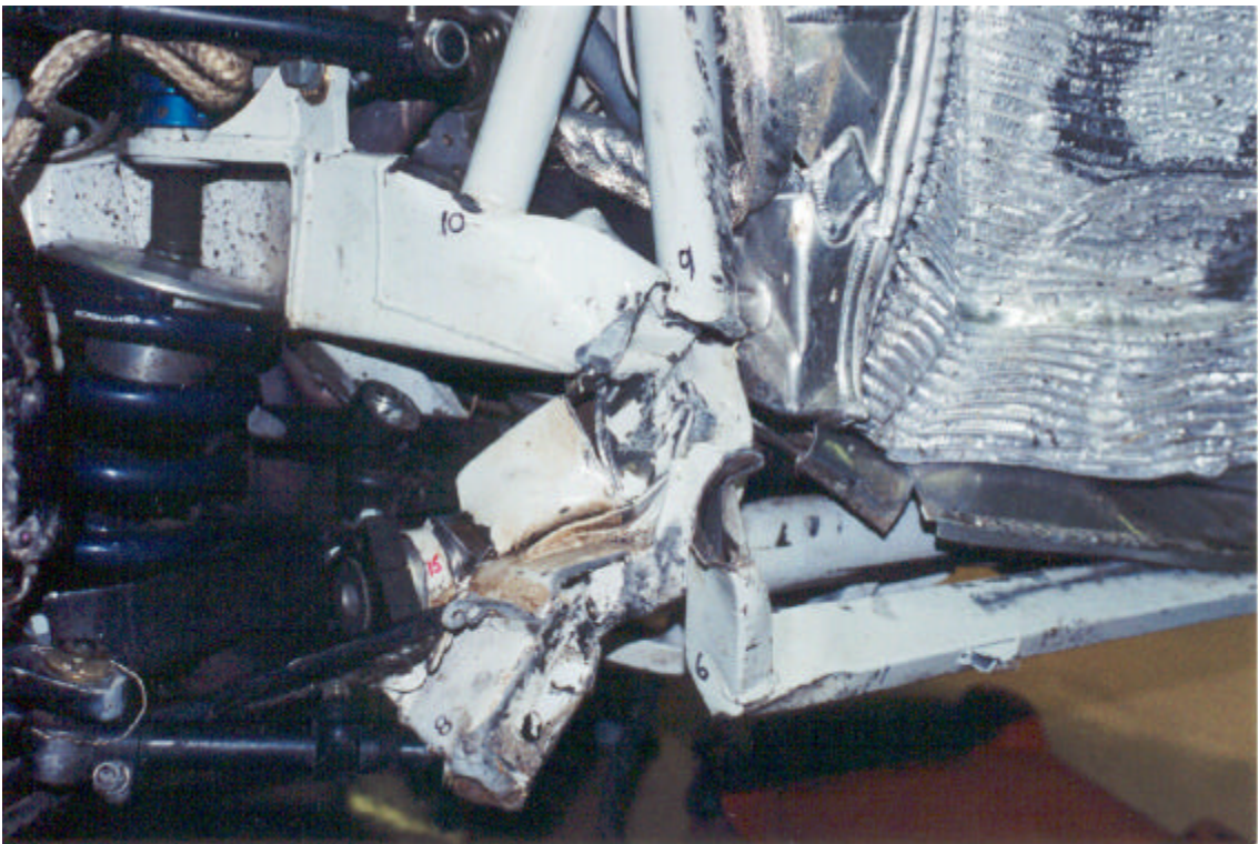
Figure 9. Right Front Damage on No. 3
