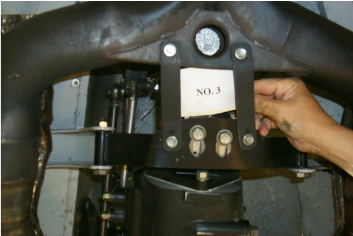
Figure 12. Rearward Movement of Transmission on No. 3 Car
