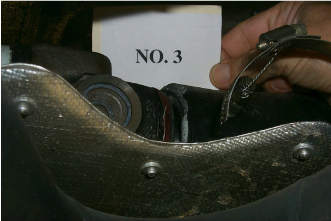
Figure 13. Deformation of Transmission Housing
